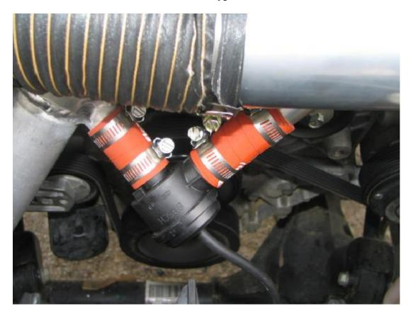
Install the orange flexible scat hose in the right position instead of the orange stick hose.
