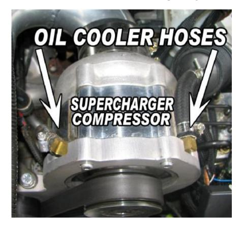
In the Photo brass fittings were used to attach the oil lines. Your kit contains banjo bolts and fittings for this step.
