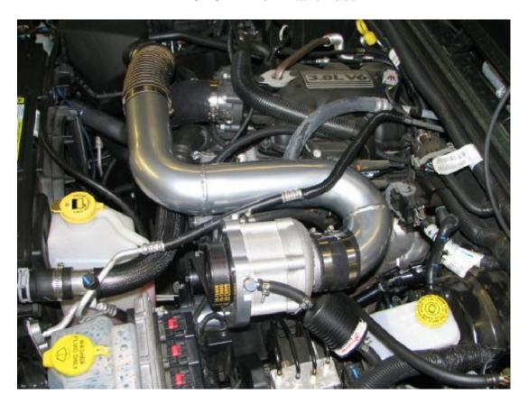
PHOTO #30 Vacuum tube & Tee to evaporator valve
