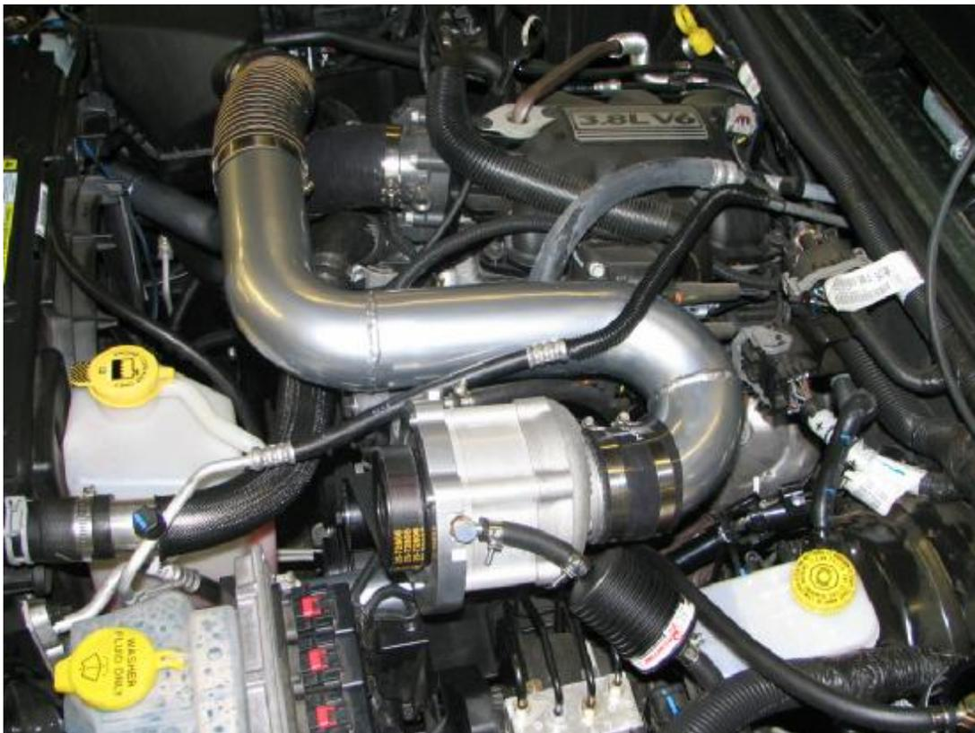
**PHOTO #30 Vacuum tube & Tee to evaporator valve**
