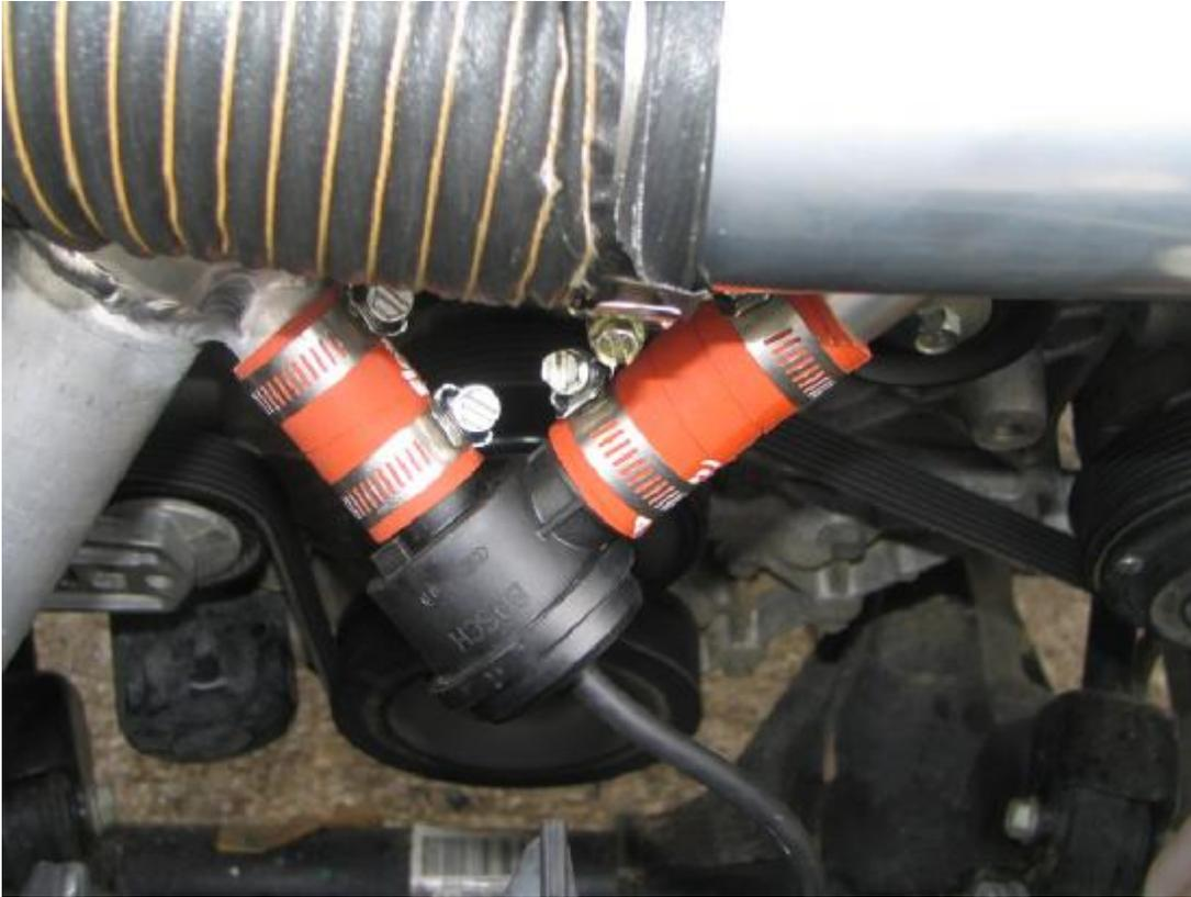
**Install the orange flexible scat hose in the right position instead of the orange stick hose.**
