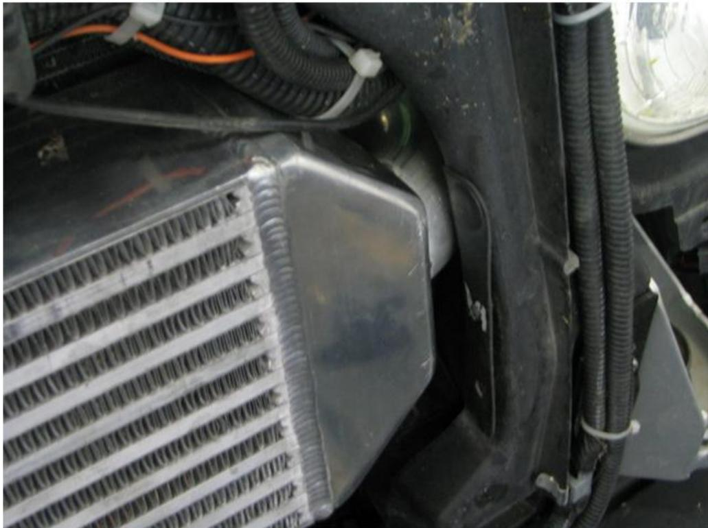
**PHOTO# 10 – Supercharger Discharge Tube Installation**
