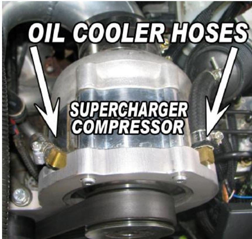
In the Photo brass fittings were used to attach the oil lines.
