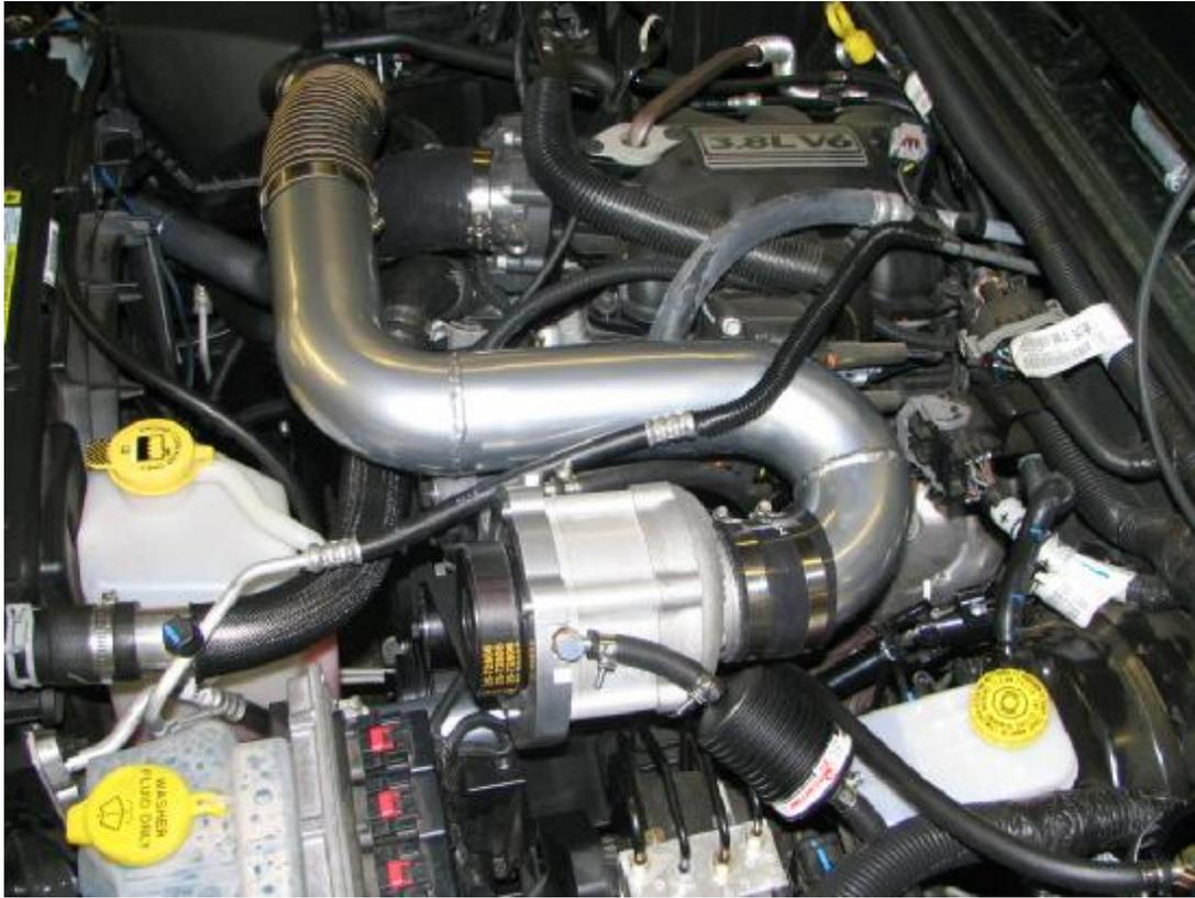
**PHOTO# 25 – Oil Cooler Hoses (at Supercharger)**
